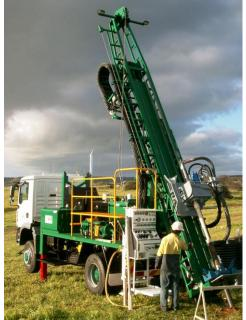
Rig 8 is the latest addition to J&S Drilling's fleet, build completed in 2009.
